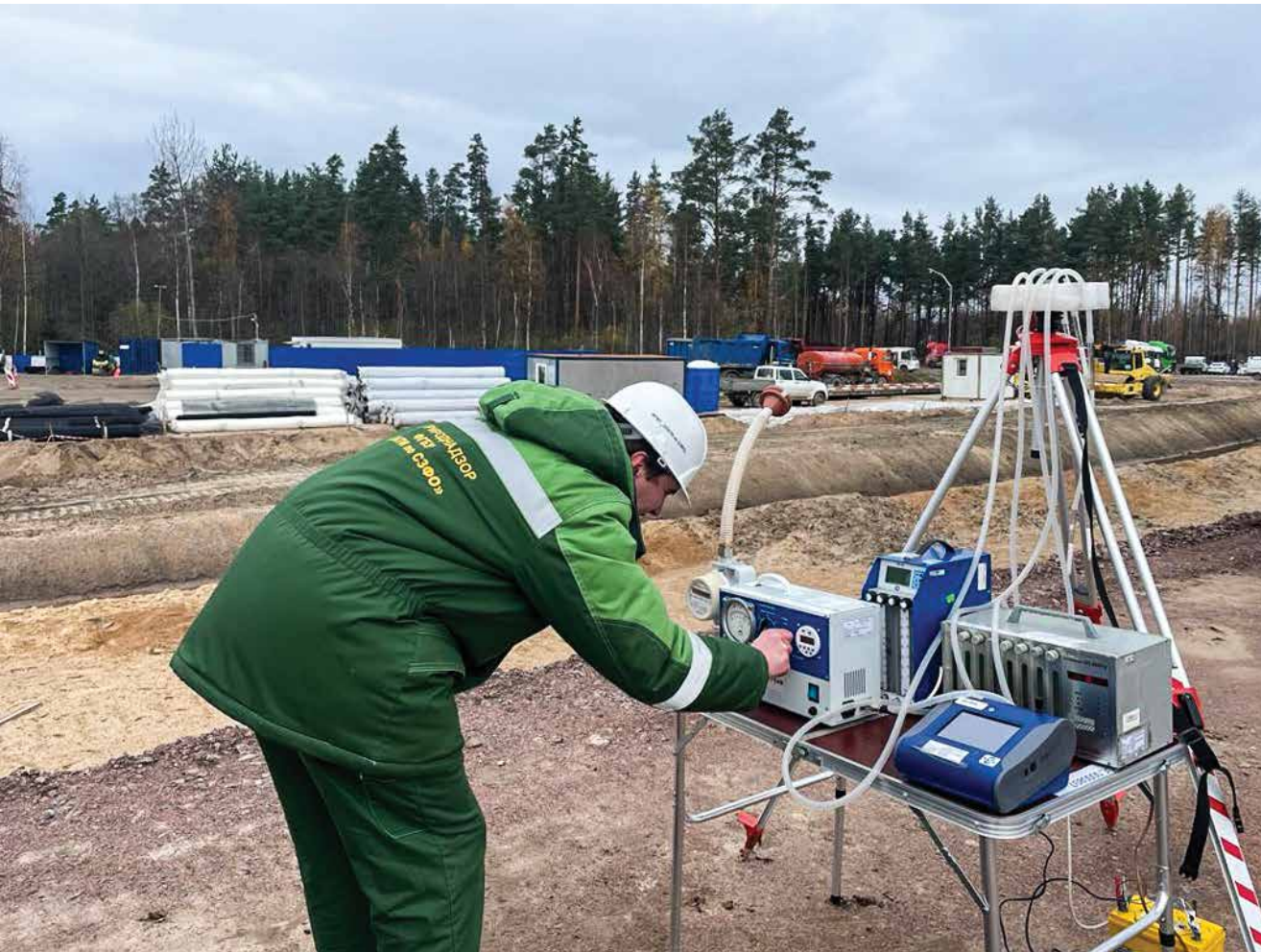
Photo 7.10.1. Air sampling and noise levels measuring
